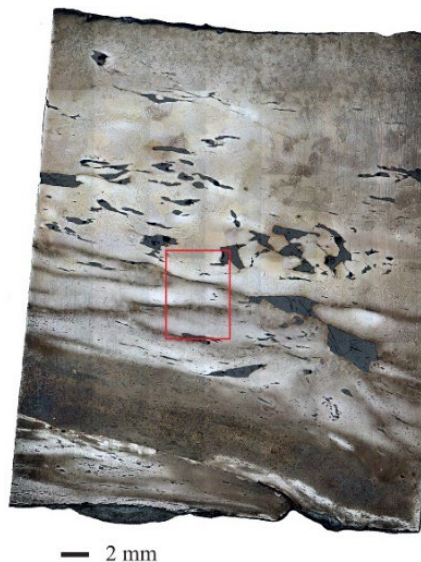
Fig.11. Notre Dame Cathedral, Paris. Oberhoffer on sample NN9-T with mesoscopic microscopic changes in P content, with highrate in lighter areas. [18]
