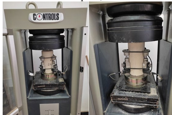
Figure 3 : Device for determining the stress-strain diagram of samples with extensometers
