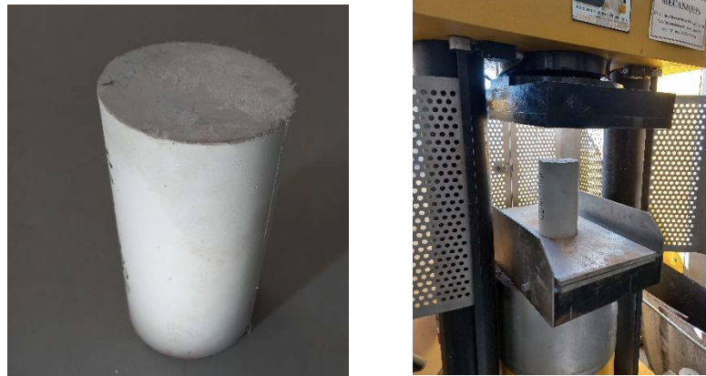
Fig. 1. Concrete specimens prepared for compressive strength test.
