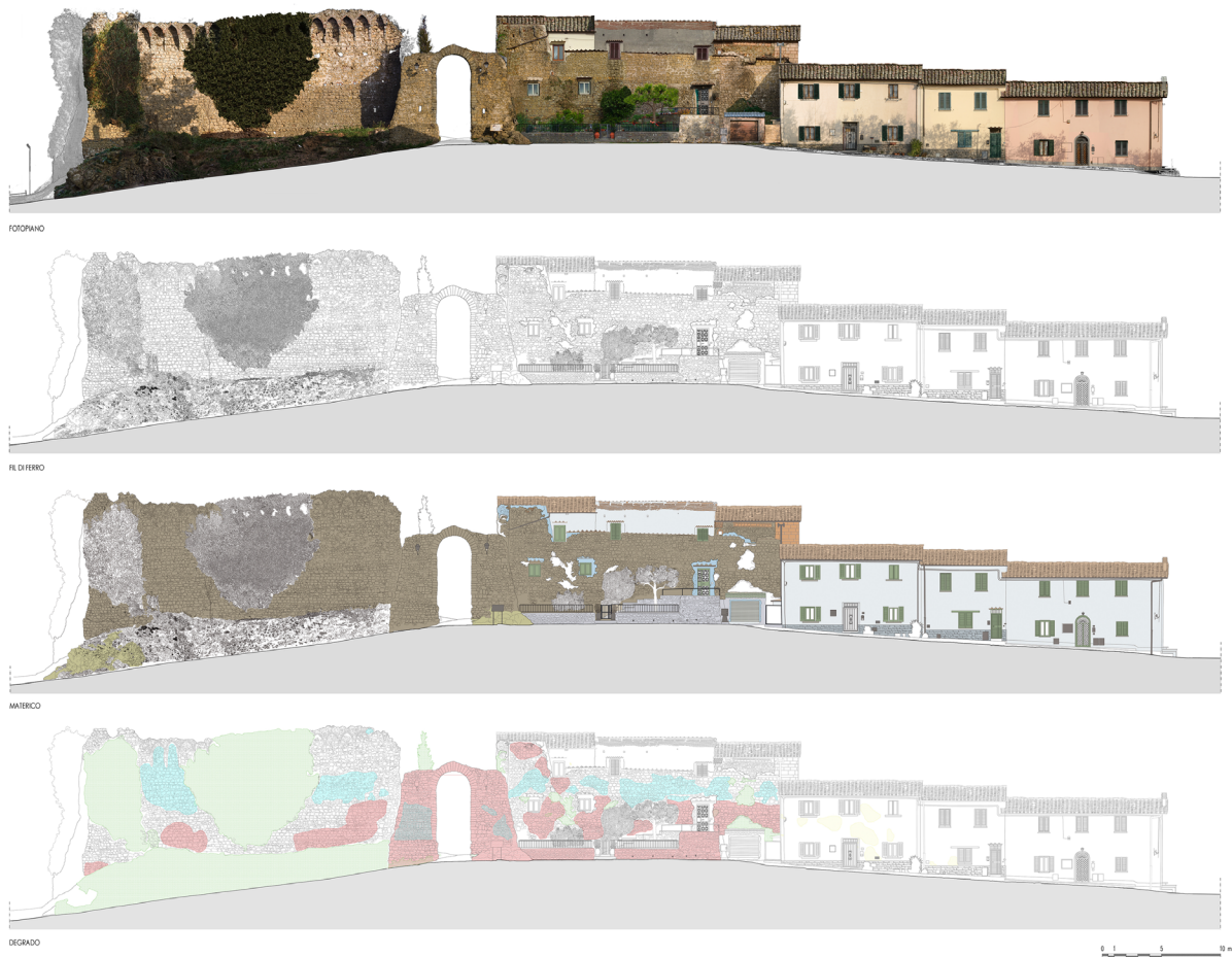
Figure 6. Front of the West Front (D-D' section) of the Fortress of Malmantile, from top to bottom, Photoplane, Wirfreme, Material Analysis and the state of conservation.
