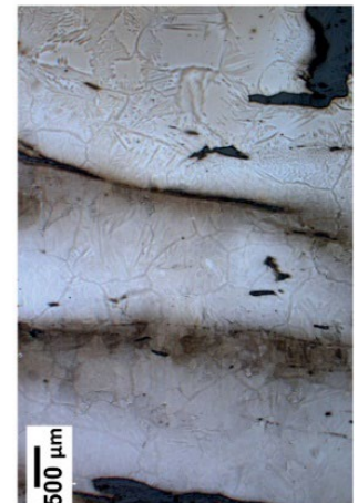
Fig.11. Notre Dame Cathedral, Paris. Oberhoffer on sample NN9-T with mesoscopic microscopic changes in P content, with highrate in lighter areas. [18]
