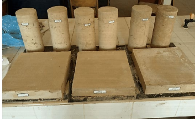
Fig.4. Bricks prepared after demolition.
