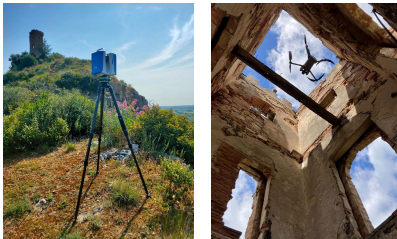
Fig. 2, On the right, the cliff where the Caprona tower stands, and the scanner used is the Z+Inager 5016.
