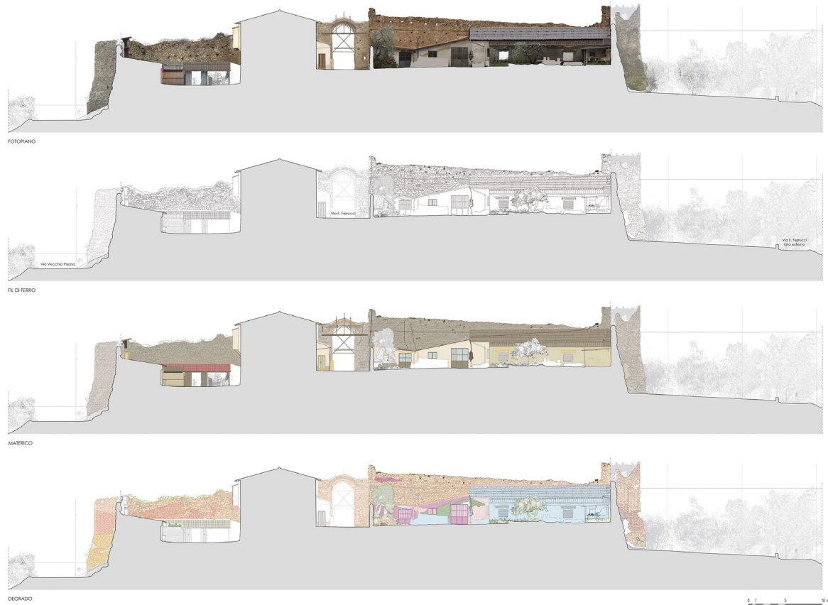
Figure 7. An internal cross section (H-H' section), of the Fortress of Malmantile, from top to bottom, Photoplane, Wirfreme, Material Analysis and the state of conservation.
