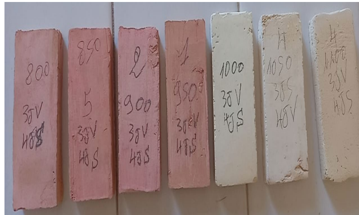
Figure 10: sintered bricks at different temperatures
