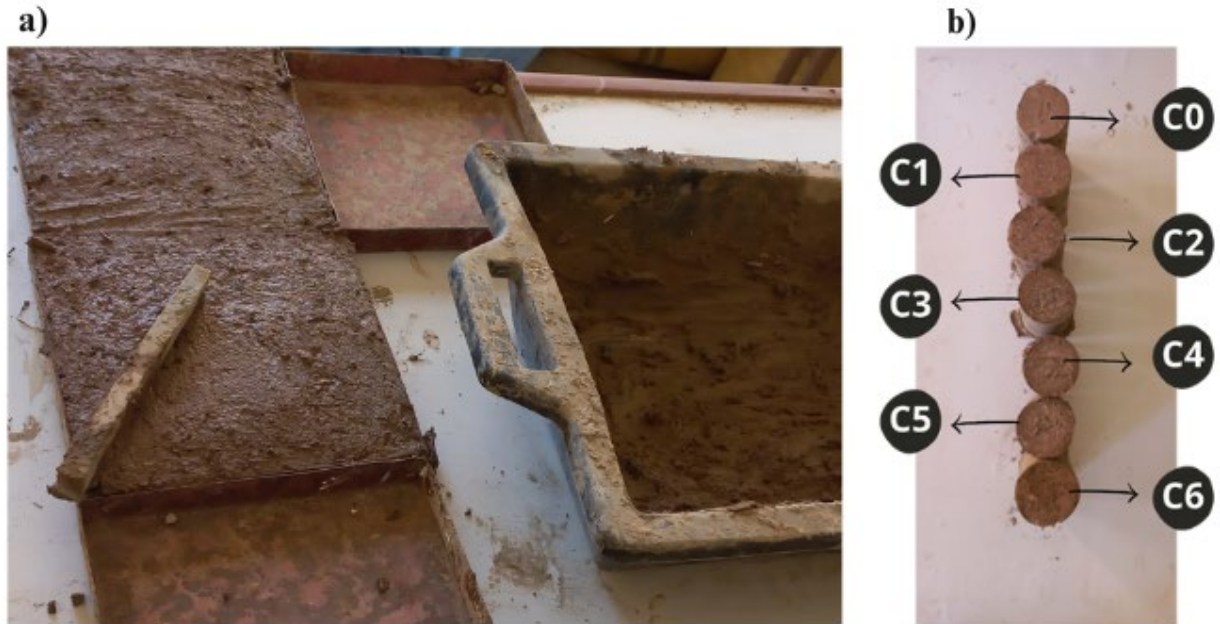
Fig 3. Samples preparation, a for thermal tests, b for mechanical tests
