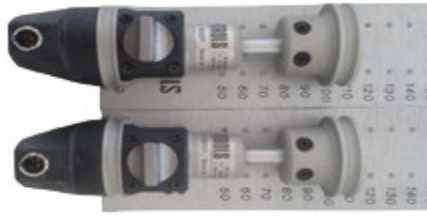
Figure 4 : Longitudinal displacement measuring device (extensometers)
