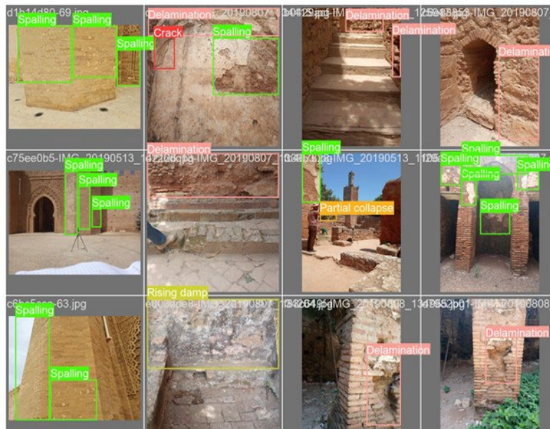
Fig. 3. Illustrative instance showcasing predicted bounding boxes utilizing the YOLOv5 model.
