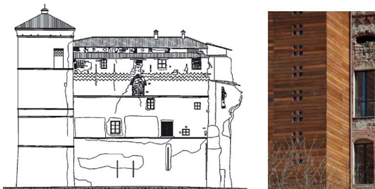
Fig.7. Saliceto Castle, Cuneo, Italy: a. East elevation, state of the places, b. Detail of technological tower reconstruction. [16]
